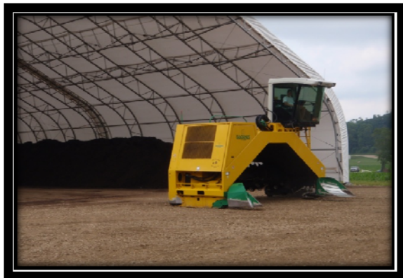
A windrow turner and the roofed composting complex at the Laurelbrook Farm
